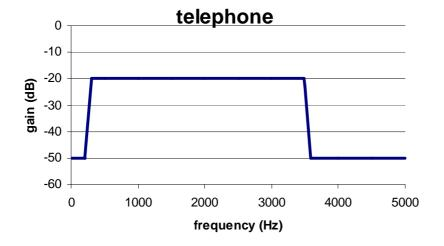
Draw correct frequency response of the telephone system.
